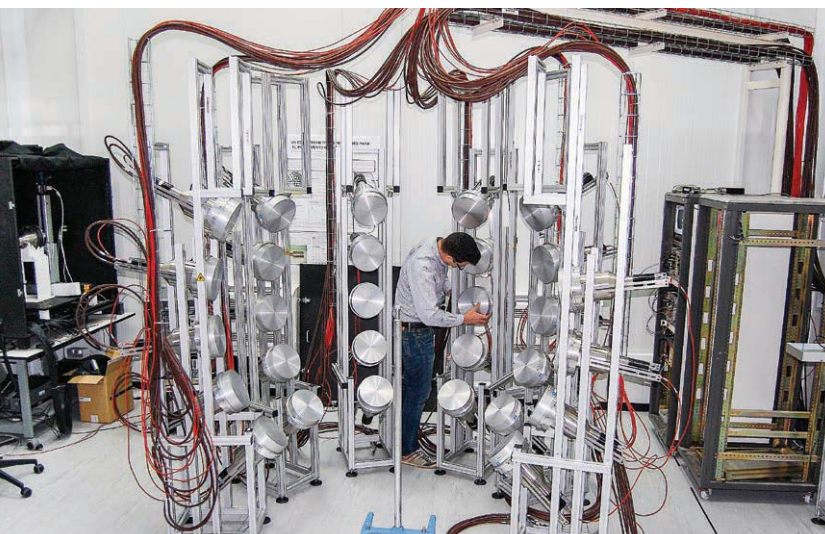
MOdular Neutron SpectromETER (MONSTER) for neutron spectroscopy studies. Part of the detectors have been built by CIEMAT and the Spanish company Scientifica Internacional S.L.
