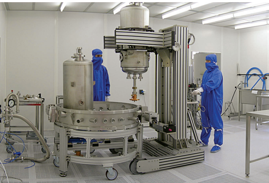
Mounting of a SPIRAL2 cryomodule in the clean room
